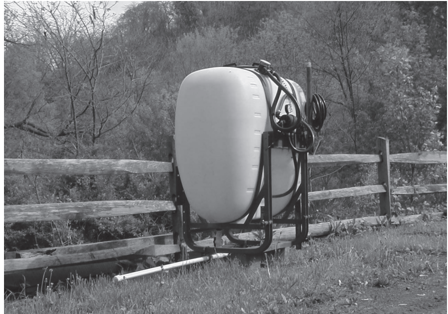
Figure 4. A tractor- or pickup-mounted water spray tank is a way to partially automate wetting arena surface materials.
