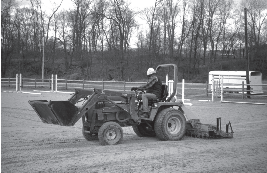
Figure 7. Equipment will be needed for frequent conditioning of the riding surface to redistribute footing for an even coverage of the base material and, in some cases, to loosen compacted surface materials.
